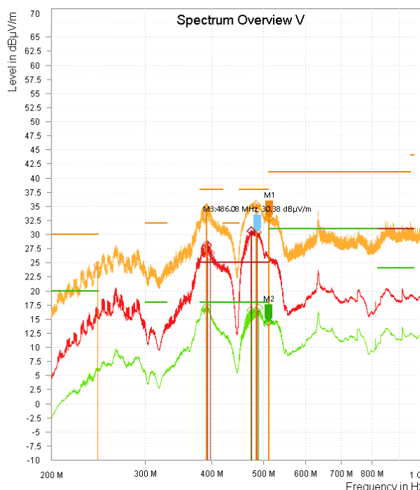
Figure 3-4. TPSM33620-Q1 Radiated EMI without Snubber, Vertical Polarization, 12VIN, 3.3VOUT, 2A
