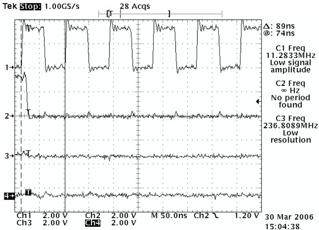
Figure 6. Four AIC33 Devices TDM Bus (Details on BCLK)
