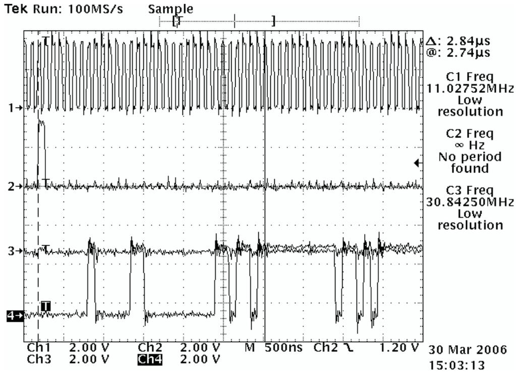
Figure 5. Four AIC33 Devices TDM Bus (Details Within the First AIC33)
