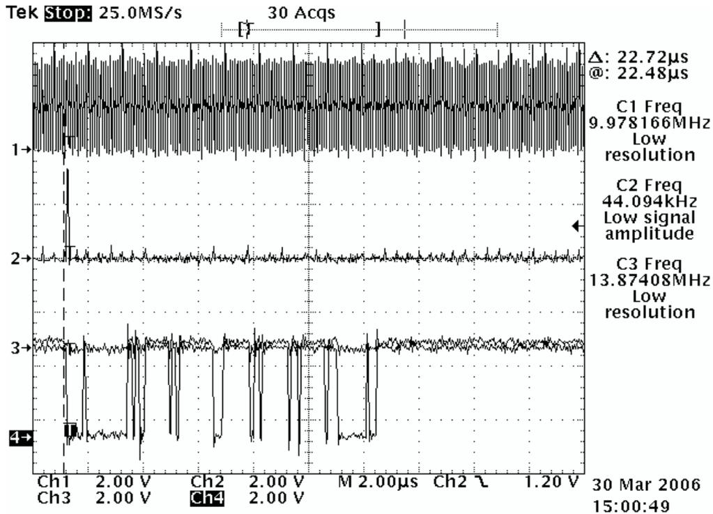
Figure 4. Four AIC33 Devices TDM Bus (Details Within a Frame)
