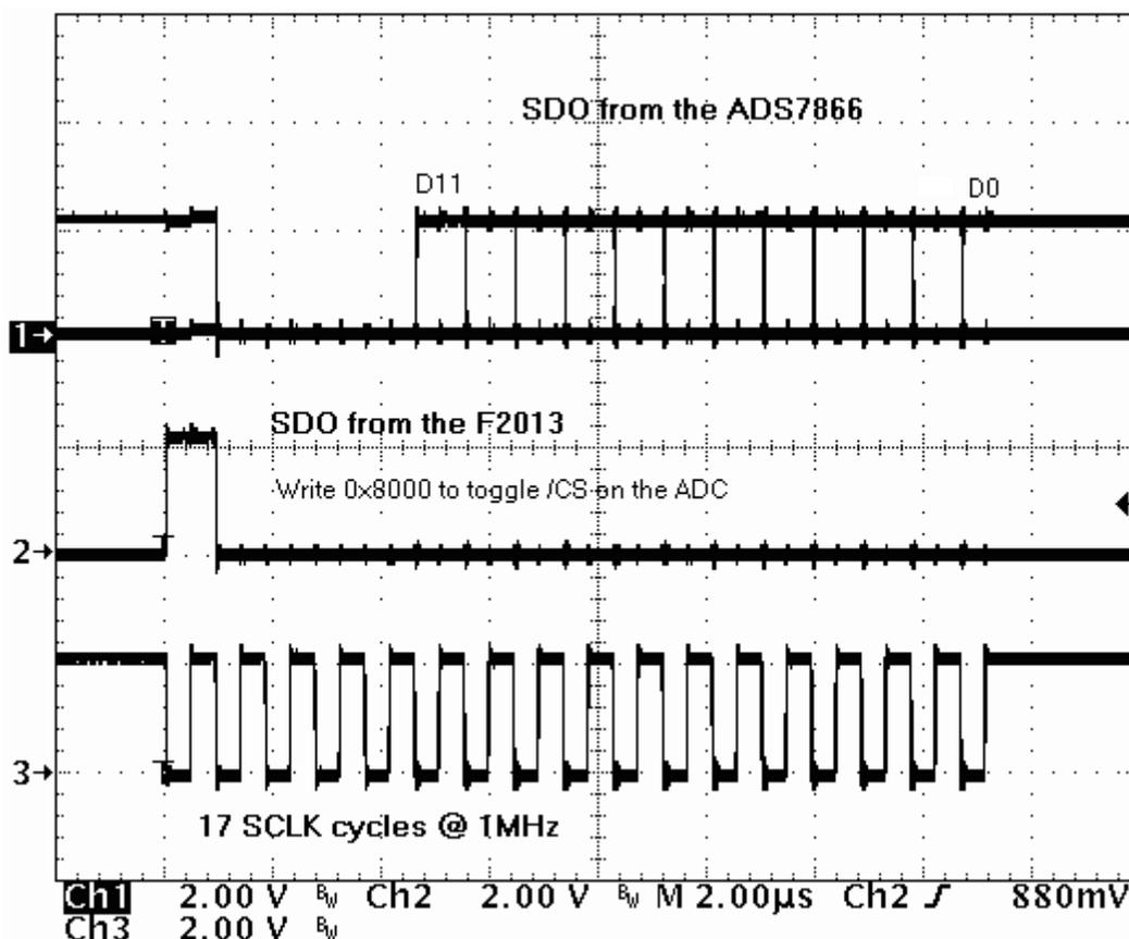
Figure 2. Complete Conversion Cycle – Single Channel
