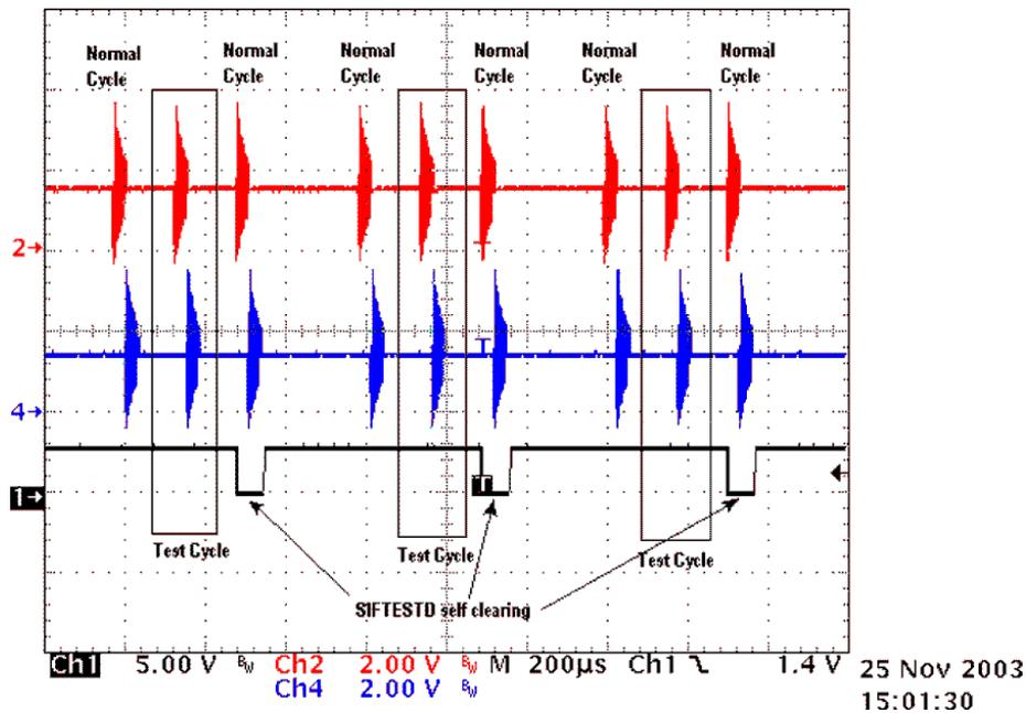
Figure 3. TCI LC Sensor Example
