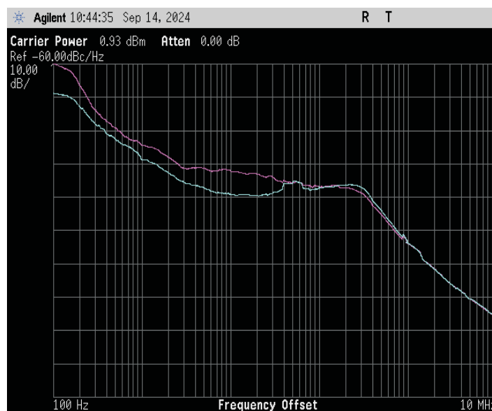
Figure 4. Phase Noise Comparison With TCXO vs TRF3750 and VCXO as Reference
