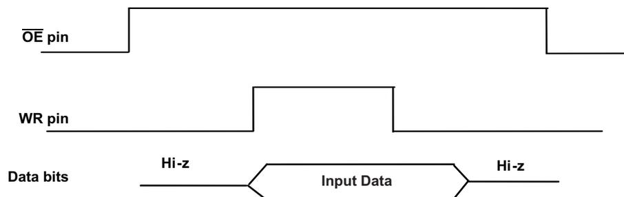
Figure 2. THS1041 Register-Writing Logic Timing
