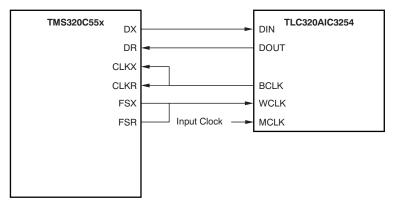
Figure 1. McBSP Connection to TLV320AIC3254 Codec
