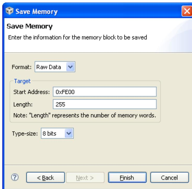
**Figure 8. Save Device Memory Content to a File in CCS**
