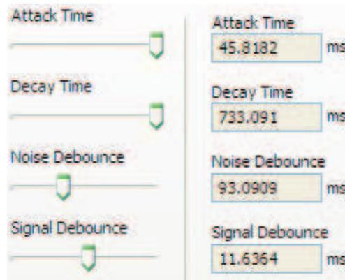
**Figure 9. Attack, Decay and Debounce Controls and Indicators**
