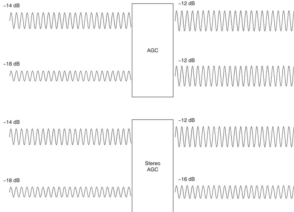
Figure 1. Stereo AGC Operation
