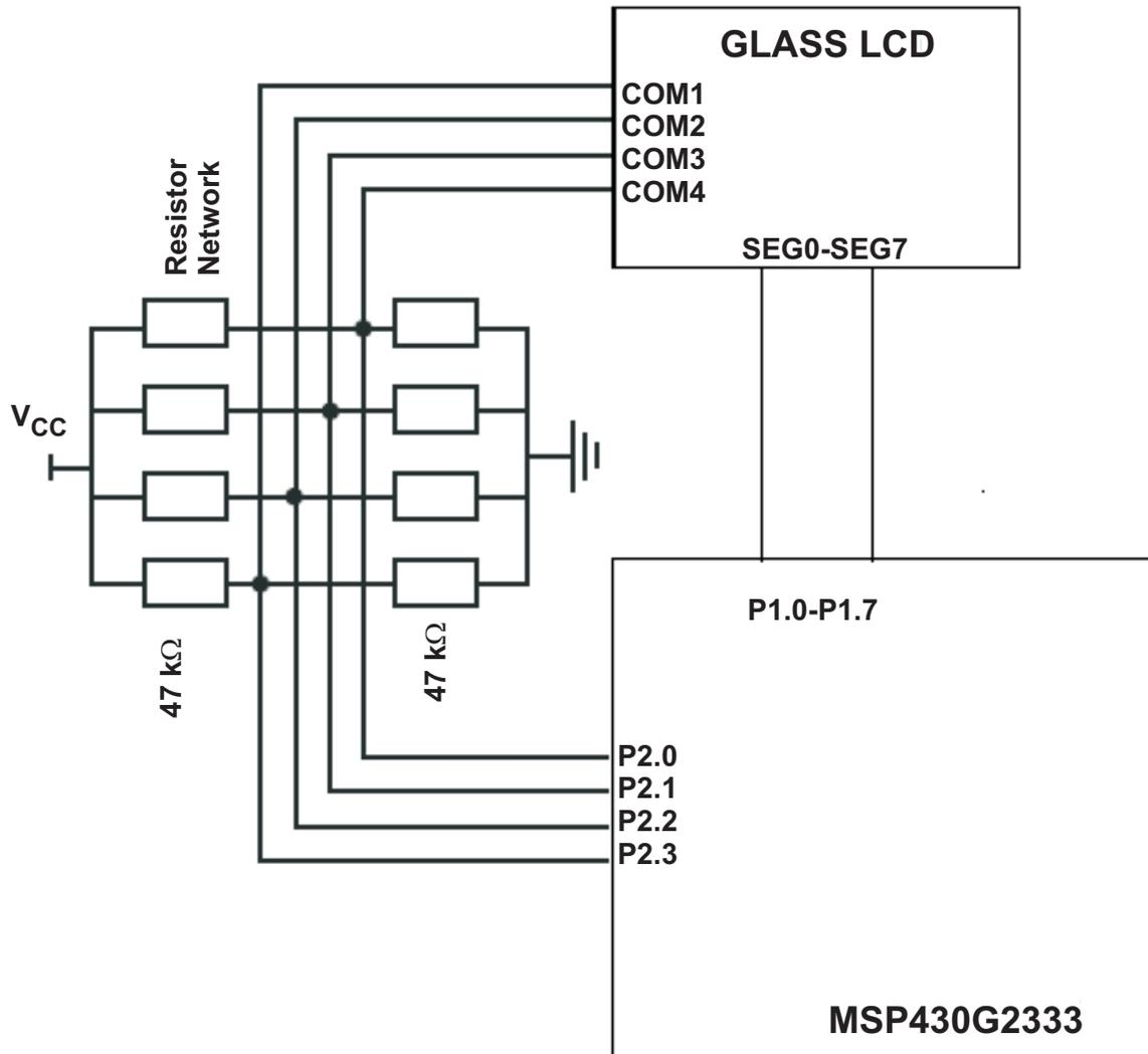
Figure 4. Glass LCD Connections to MSP430G2333 Device
