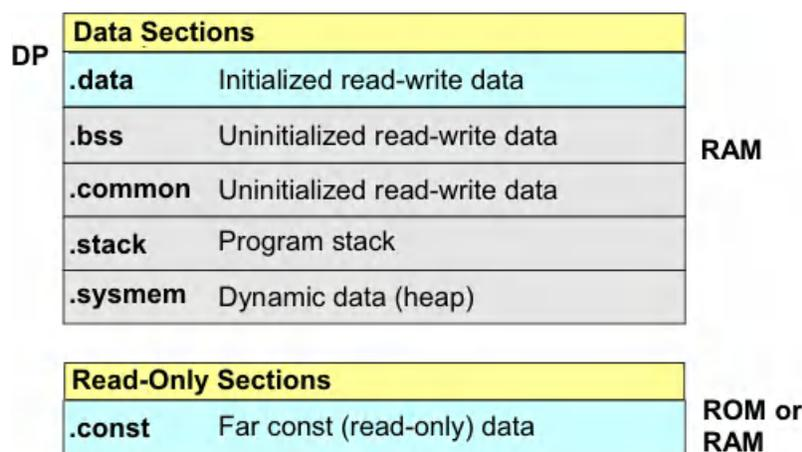
**Figure 4-1. Data Sections and Segments (Typical)**
