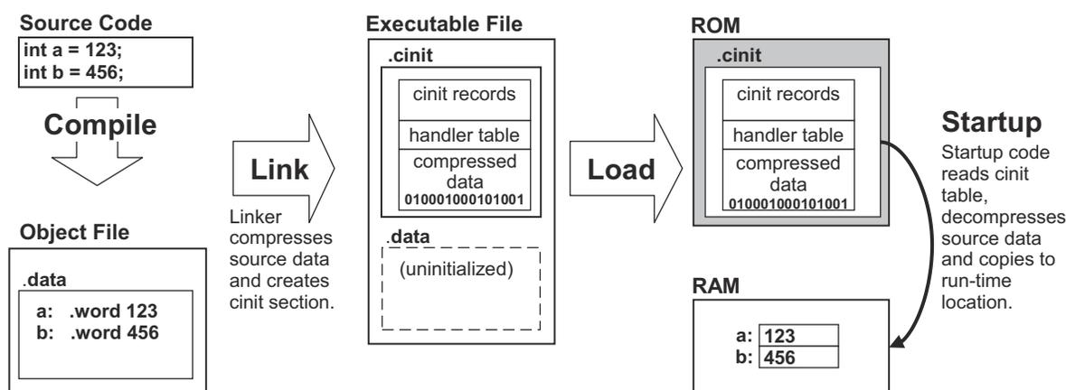
**Figure 14-3. ROM-Based Variable Initialization Via cinit**
