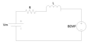
Figure 1-1. BLDC Motor model
