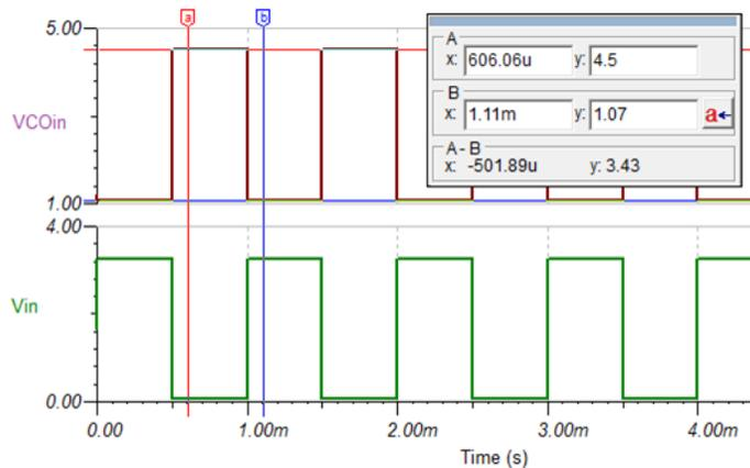
Figure 10. Simulated Waveforms of Level-Shifter Circuit using LP211
