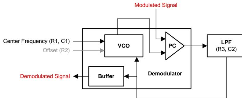
**Figure 5. Basic Block Diagram of PLL as Demodulator**
