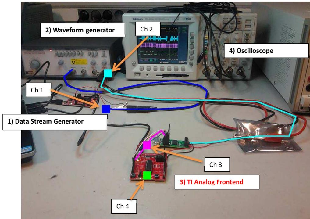
Figure 11. Test Setup
