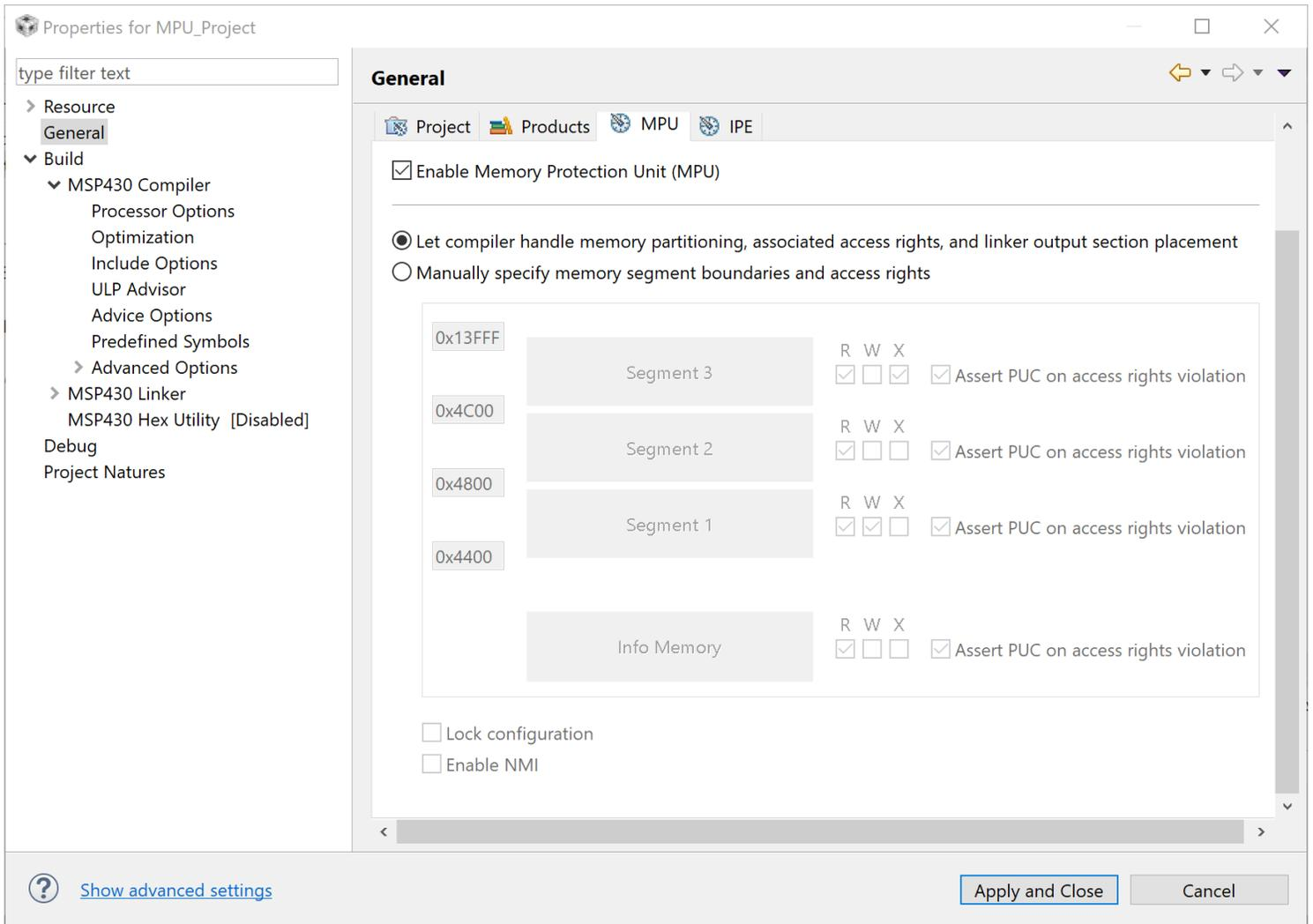
**Figure 6-4. MPU Wizard Under CCS Project Properties**
