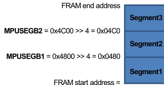
**Figure 6-2. Address to be Written in MPUSEGBx Registers**
