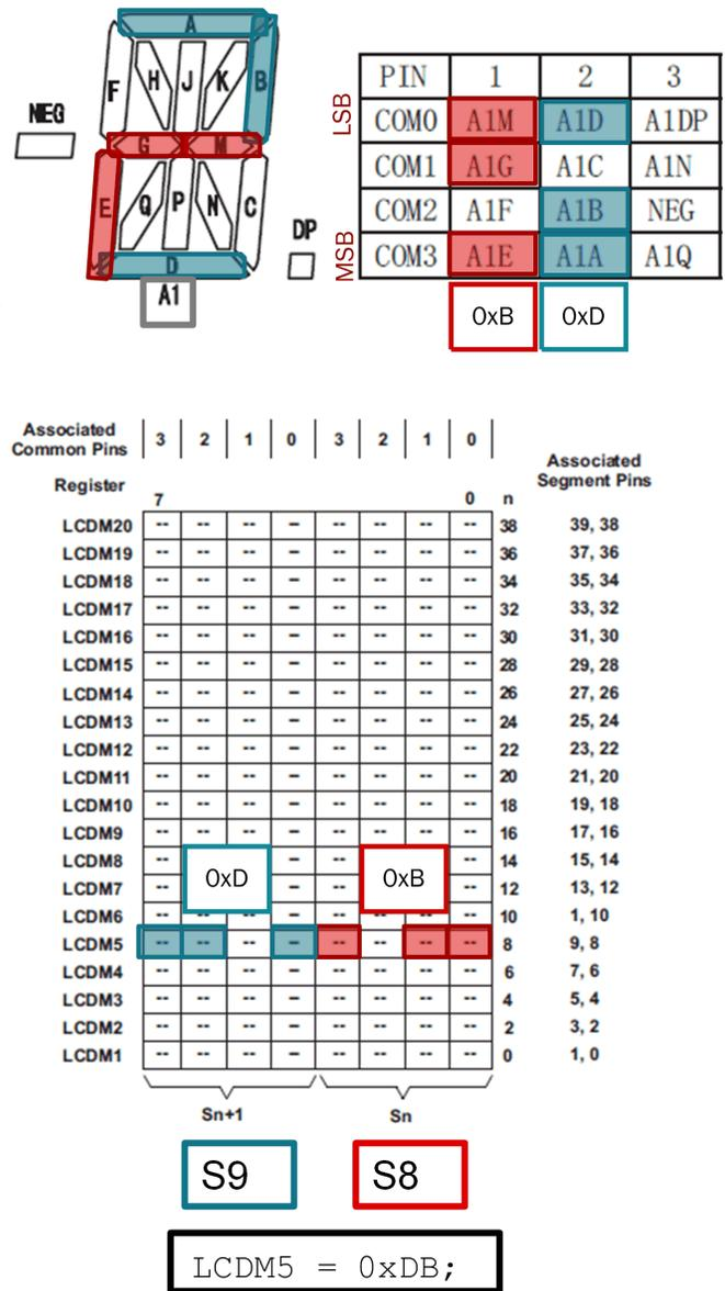
Figure 17. Example Displaying the Digit "2" Using LCD Memory (Without Special Software Techniques)
