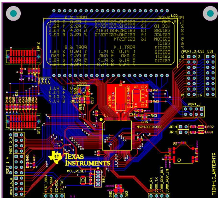
Figure 16. Portion of TIDM-LC-WATERMTR Design Showing LCD Layout
