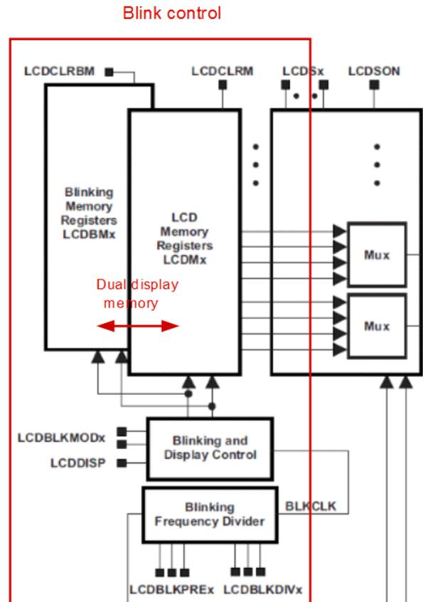
**Figure 9. LCD Blinking and Dual Display Memory**
