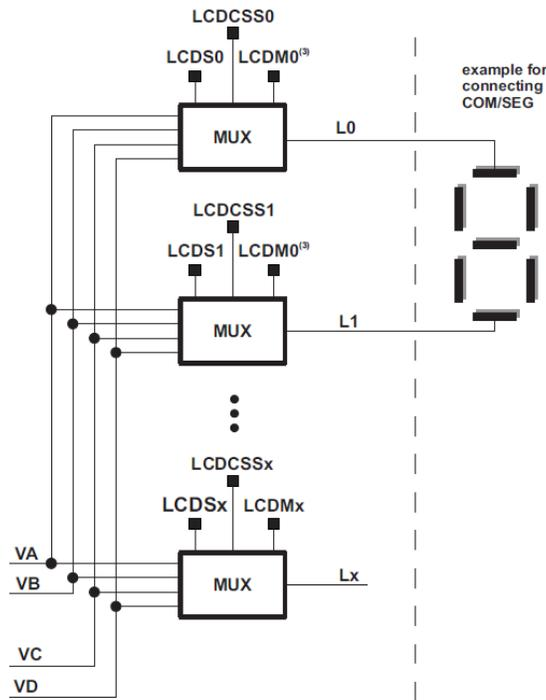
Figure 10. LCD\_E Flexible COM and SEG Configuration
