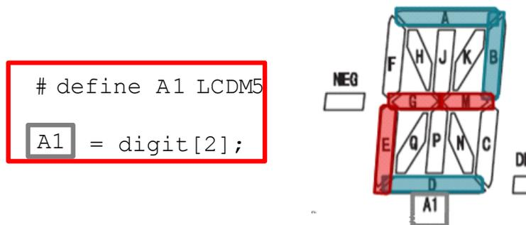
Figure 18. Using #defines for Easy-to-Read LCD Code
