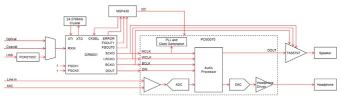
Figure 7. Hardware Design Block Diagram
