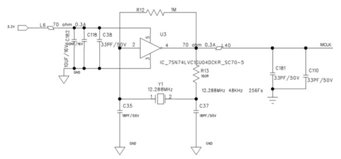
Figure 3. Crystal MCLK Generation Circuit
