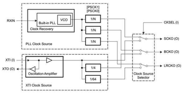
Figure 2. DIR9001 Internal Clock Tree
