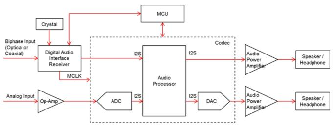
Figure 1. Traditional Digital Audio System Block Diagram
