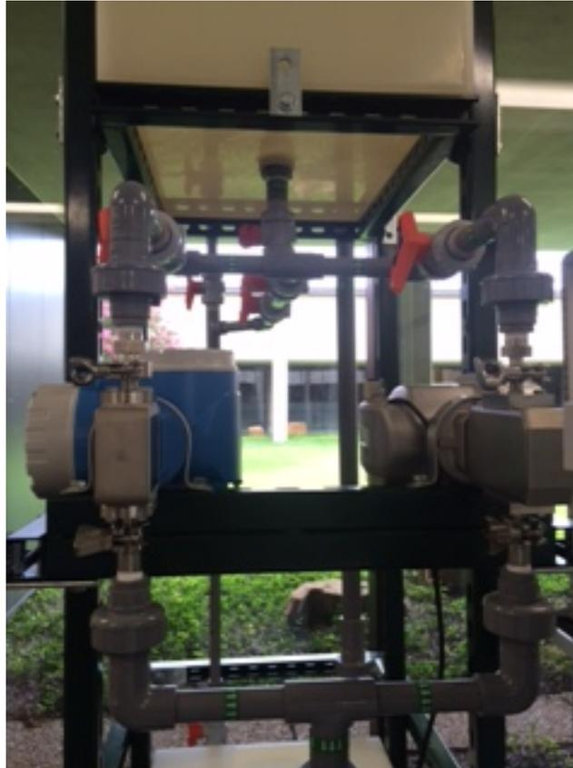
NOTE: Left arm: 0.005 to 0.35 GPM; right arm: 0.25 to 8 GPM
