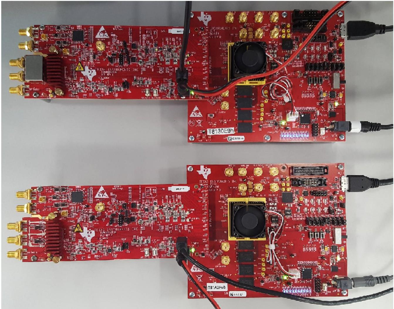
**Figure 2. TSW40RF82 and TSW14J56 Setup**
