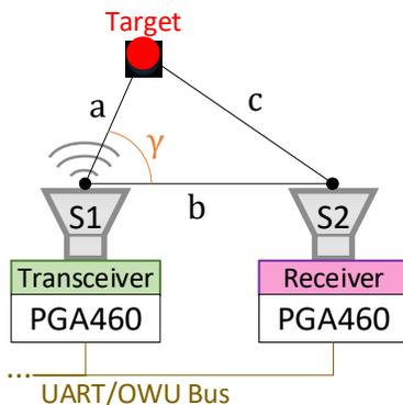
Figure 2. Triangulation Block Diagram Solution for a Transceiver and Receiver Combination
