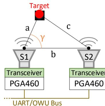
Figure 3. Triangulation Block Diagram Solution for a Multi-Transceiver Combination
