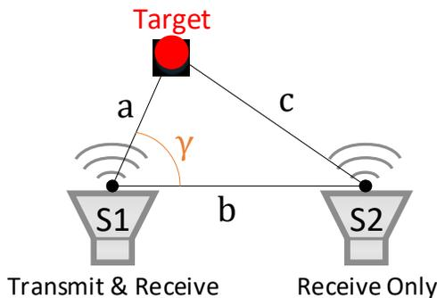
Figure 1. Simplified Ultrasonic Time-of-Flight Concept
