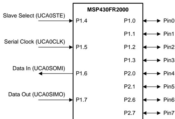
**Figure 1. SPI I/O Expander Block Diagram**
