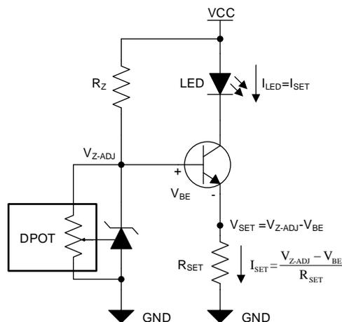
Figure 1. DPOT Based Biasing
