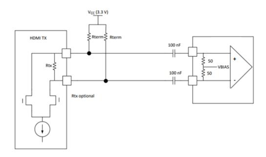
Figure 1. External Termination Network for AC-coupled Interface
