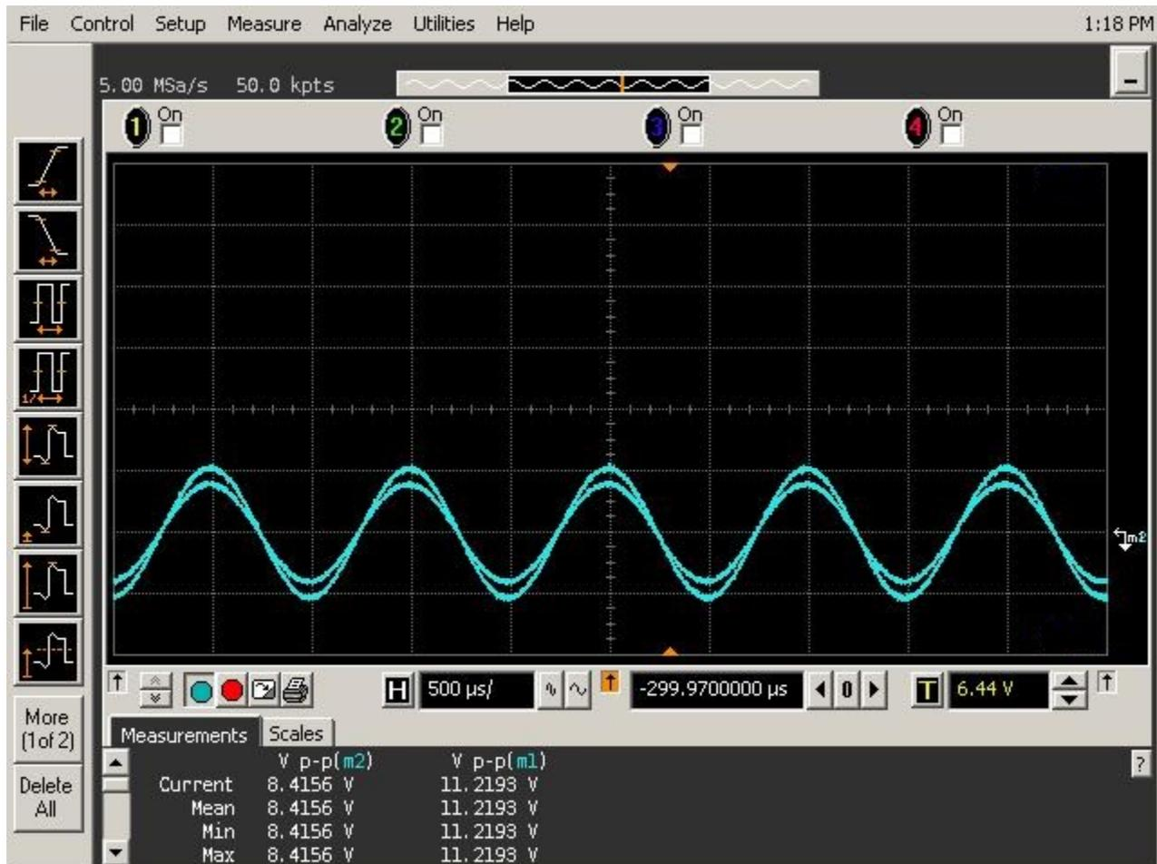
Figure 8. Output Waveforms - Thermal Foldback
