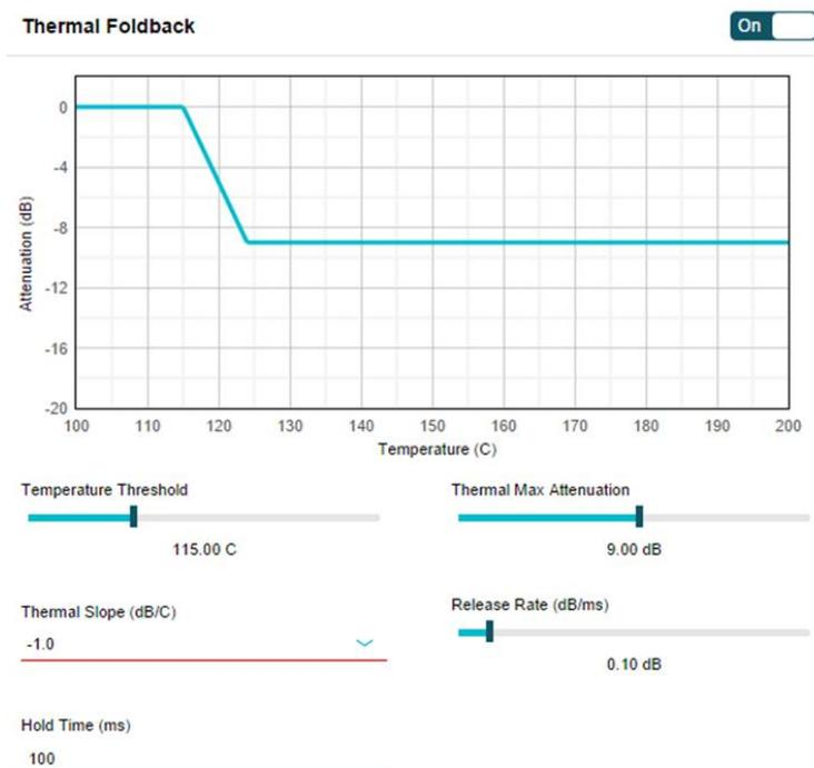
Figure 1. Thermal Foldback Control Panel
