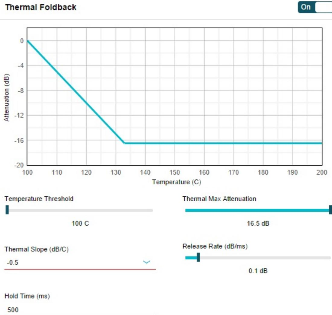
**Figure 2. Thermal Foldback Settings**
