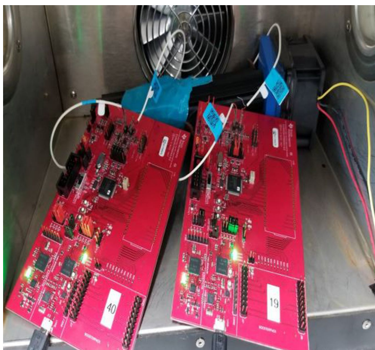
Figure 3-3. Comparative Testing of Transducer Pairs Setup
