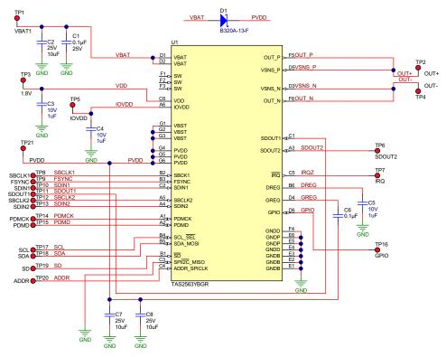
Figure 2-1. External PVDD Schematic
