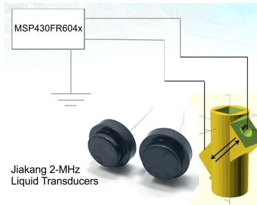
**Figure 2-2. Jiakang 2-MHz Ultrasonic Configuration**
