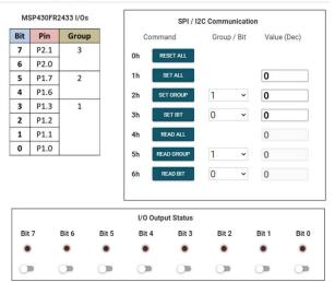
Figure 3. SPI I/O Expander GUI
