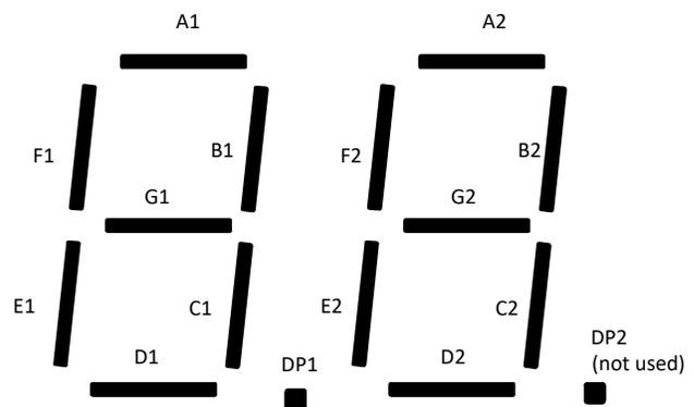
Figure 2. 2-Digit, Common-Anode 7-Segment LED Display Top View
