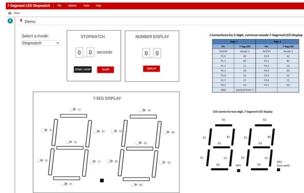
**Figure 4. 7-Segment LED Stopwatch GUI**
