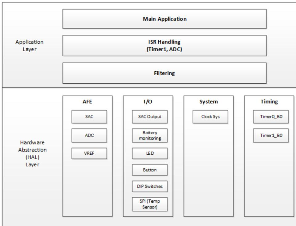
**Figure 2-1. Software Architecture**
