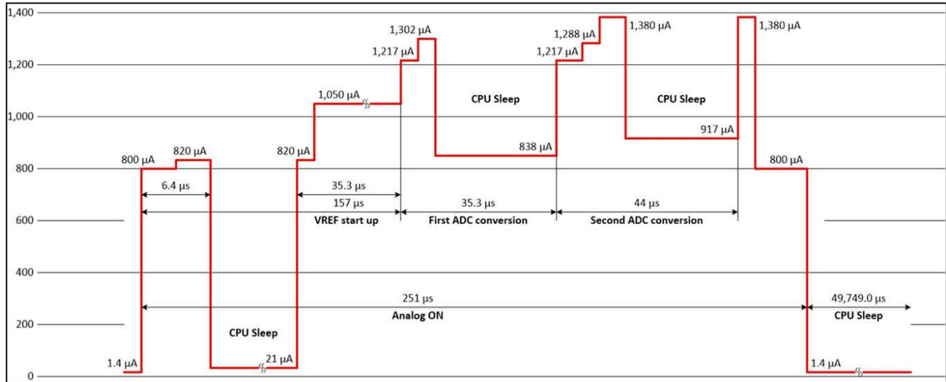
Figure 2-3. Power Profile of MSP430 PIR Demo Software
