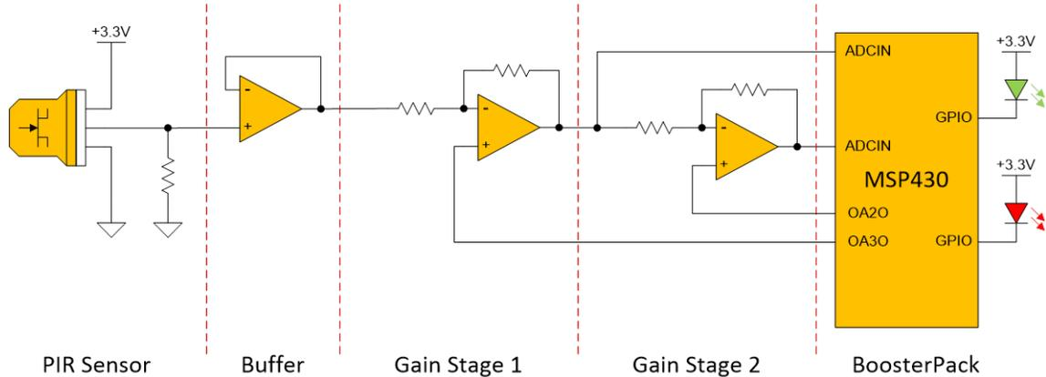
Figure 1-6. Capacitor Free Signal-Chain
