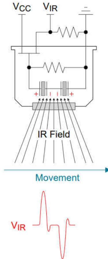
**Figure 1-2. PIR Motion Sensor Illustration**
