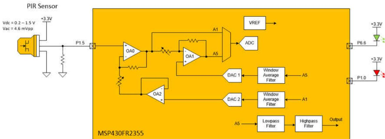
Figure 1-7. PIR Signal-Chain Integrated Into MSP430FR2355
