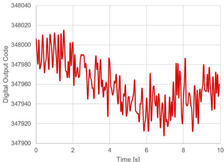
Figure 2-7. PIR Signal Ripples/Noise
