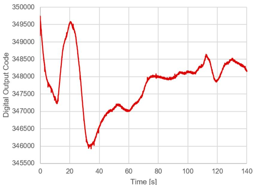
Figure 2-4. PIR Sensor Signal Drift Over Time
