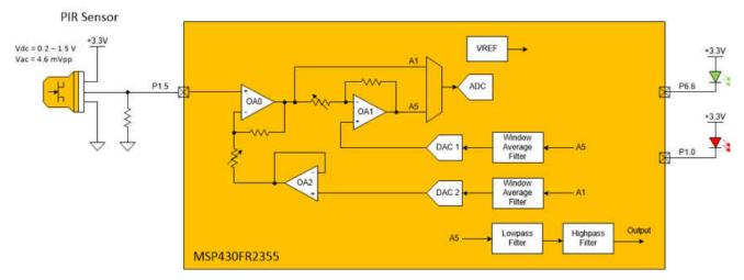
Figure 1-7. PIR Signal-Chain Integrated Into MSP430FR2355
