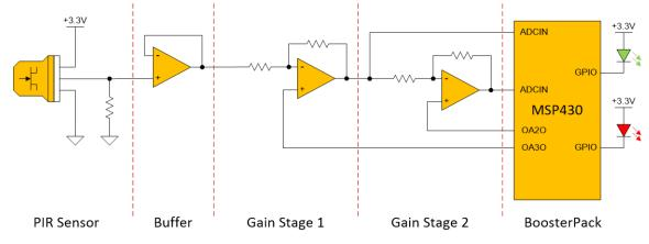
Figure 1-6. Capacitor Free Signal-Chain
