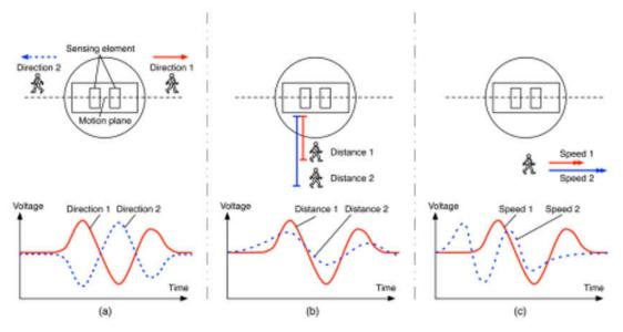
Figure 1-3. PIR Sensor Output Signal
