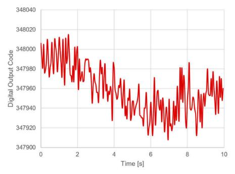
Figure 2-7. PIR Signal Ripples/Noise
