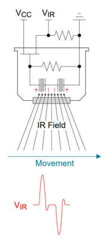
Figure 1-2. PIR Motion Sensor Illustration
