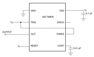
Figure 6-1. 555 Timer Configured for a Comparator with Hysteresis
