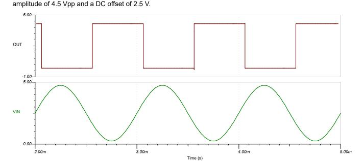
TRIG/THRESH = 4.5-Vpp 1-kHz sine wave with a 2.5-V DC offset
