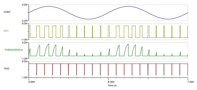
VS = 5 V,  $R_A = 12 \text{ k}\Omega$ , C = 2 nF, TRIG = 100-kHz square wave with 98% duty cycle, and CONT = 4-Vpp 1-kHz sine wave with a 2.5-V DC offset
