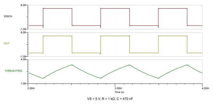
Figure 3-2. TINA-TI Simulation Results for a 50% Duty Cycle Oscillator Using a 555 Timer
