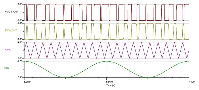
VS = 5 V, MARGIN\_HIGH\_CODE = 810, MARGIN\_LOW\_CODE = 410, CODE\_STEP = 32, SLEW\_RATE = 4  $\mu$ s/step, MARGIN\_HIGH = 4 V, MARGIN\_LOW = 2 V, VDAC = 10-kHz triangle wave, and VFB = 1.2-Vpp 1-kHz sine wave with a 3-V DC offset
