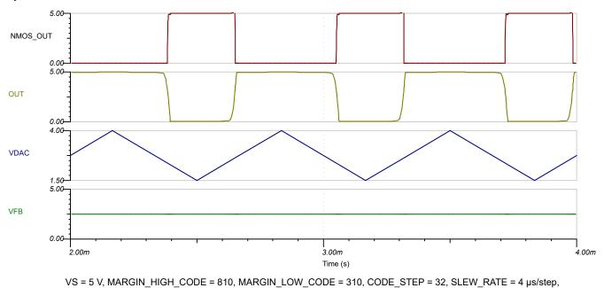
Figure 3-6. TINA-TI Simulation Results for a Variable Duty Cycle Oscillator Using a DAC53701
