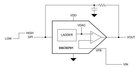
Figure 6-3. Smart DAC Configured for a Comparator with Hysteresis
