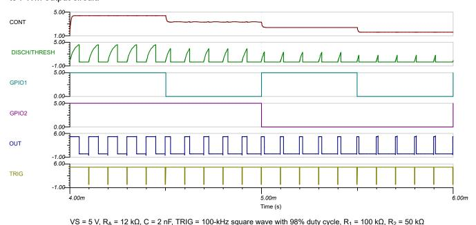
Figure 5-2. TINA-TI Simulation Results for GPI to PWM Output Using a 555 Timer
