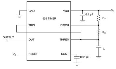
Figure 3-3. 555 Timer Configured for a Variable Duty Cycle Oscillator
