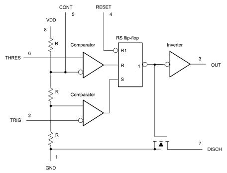
Figure 2-1. Functional Block Diagram of a 555 Timer
