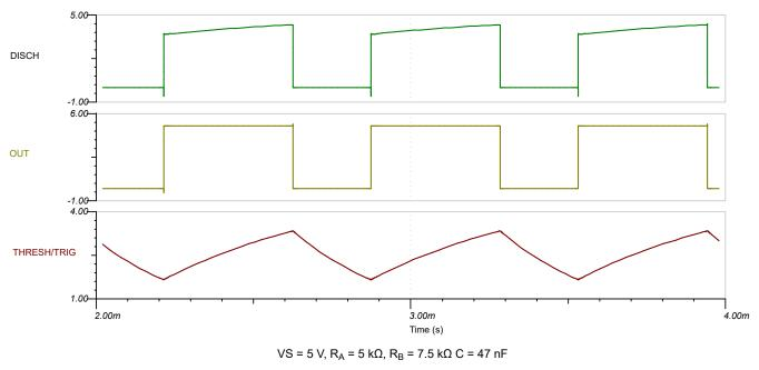
Figure 3-4. TINA-TI Simulation Results for a Variable Duty Cycle Oscillator Configuration Using a 555
