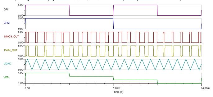
VS = 5 V, MARGIN\_HIGH\_CODE = 1023, MARGIN\_LOW\_CODE = 0, CODE\_STEP = 16, SLEW\_RATE = 4  $\mu$ s/step, MARGIN\_HIGH = 5 V, MARGIN\_LOW = 0 V, VDAC = 2-kHz triangle wave, R<sub>1</sub> = 5 k $\Omega$ , R<sub>2</sub> = 2.5 k $\Omega$ , R<sub>3</sub> = 5 k $\Omega$ , R<sub>4</sub> = 5 k $\Omega$
