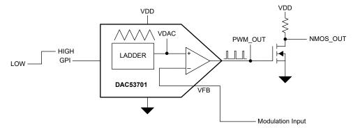
Figure 4-3. DAC53701 Configured for PWM
