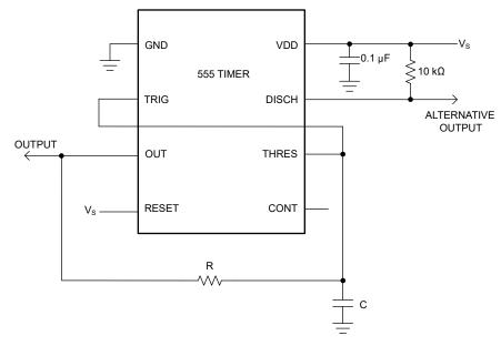
Figure 3-1. 555 Timer Configured for a 50% Duty Cycle Oscillator
