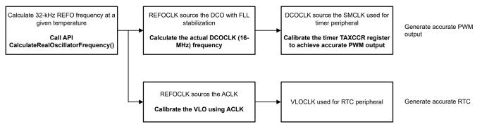
Figure 3-1. Software Flow for Achieving Improved PWM and RTC Accuracy
