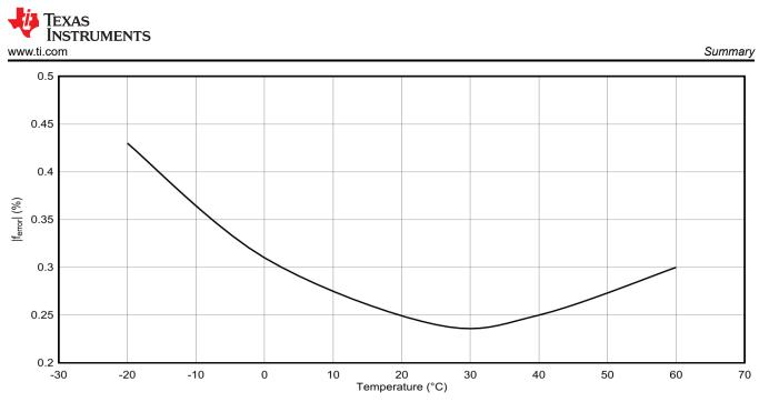
Figure 3-2. Calibrated 44-kHz Timer PWM Error Magnitude
