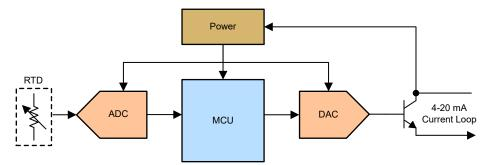
Figure 1. Typical Block Diagram of RTD Temperature Transmitter
