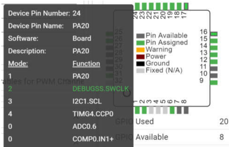
Figure 4-2. Sysconfig MCU View
