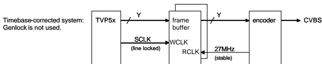
**Figure 9. TVP5146 to Time Base Corrector to Encoder – GLCO Not Required**
