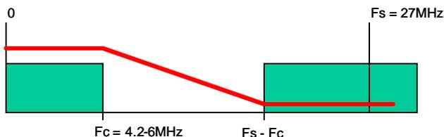
**Figure 3. Anti-Aliasing – Frequency Response**
