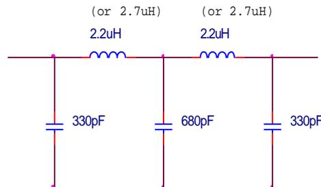
**Figure 4. Anti-Aliasing Filter Example Circuit**
