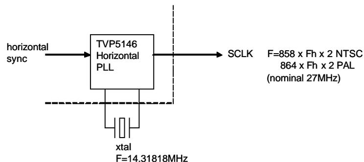
**Figure 10. Line-Locked Sampling**
