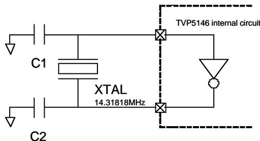
**Figure 5. TVP5146 Crystal Circuit**
