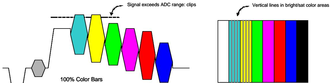
**Figure 6. Faint Vertical Lines in 100% Color Bar**
