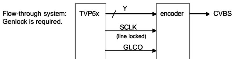
**Figure 8. TVP5146 to Encoder Flow Through System – GLCO Required**
