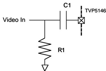
**Figure 2. Recommended Analog Input Circuit**
