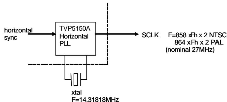
**Figure 9. Line-Locked Sampling**
