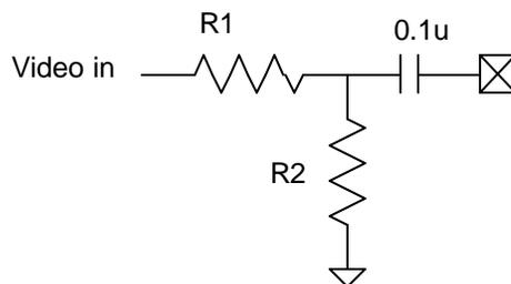
**Figure 2. TVP5150A Input Termination**
