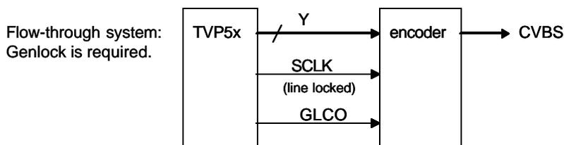
**Figure 7. TVP5150A to Encoder Flow Through System – GLCO Required**
