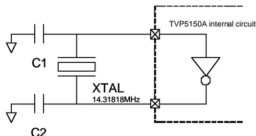
**Figure 5. TVP5150A Crystal Circuit**
