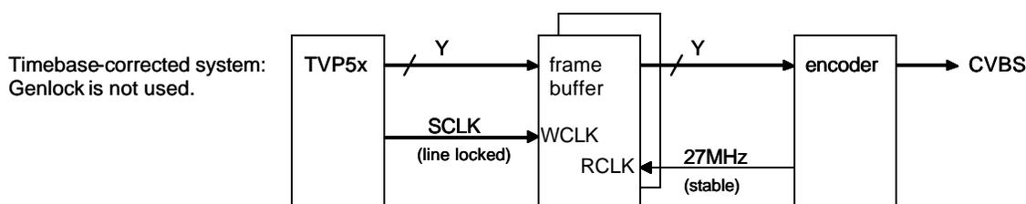
**Figure 8. TVP5150A to Time Base Corrector to Encoder – GLCO Not Required**
