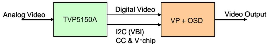
**Figure 10. Example System Interface Using the VDP**
