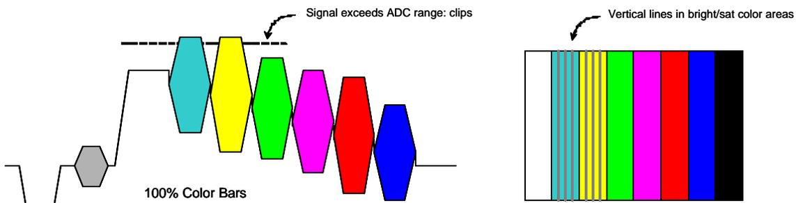
**Figure 6. Faint Vertical Lines in 100% Color Bar**
