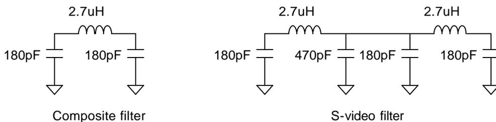
**Figure 3. Example Anti-Alias Filters for Composite and S-Video**
