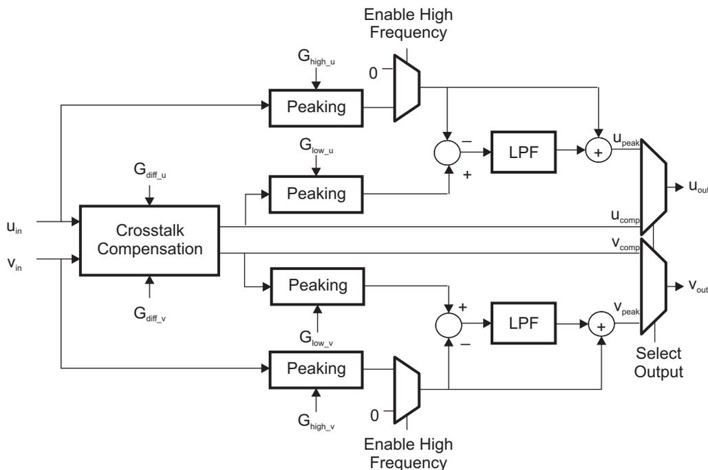
Figure 1. IF Compensation Block Diagram
