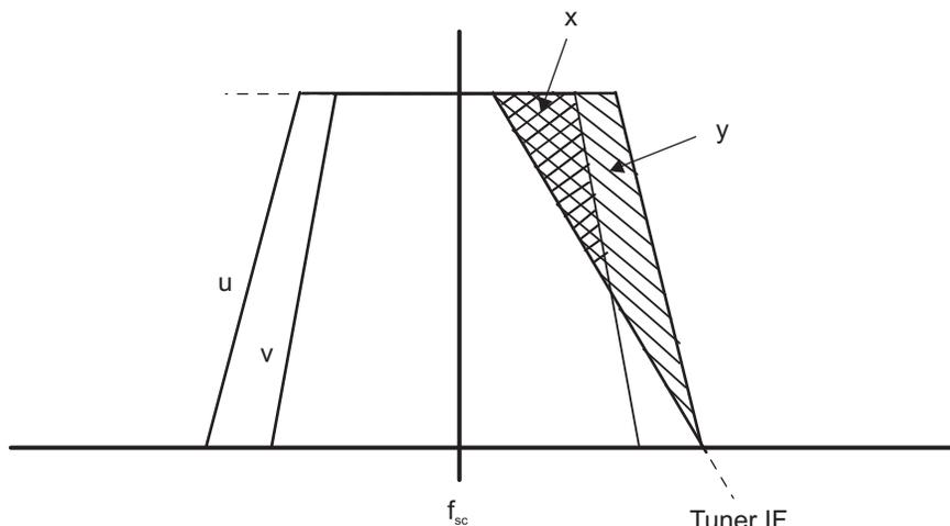
Figure 5. UV Frequency Spectrum (u Bandwidth Greater Than v)
