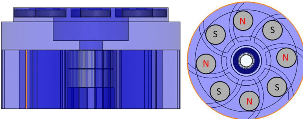
**Figure 3-3. Magnet Installation**
