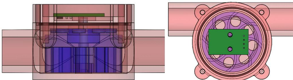
**Figure 3-7. Horizontal PCB Mount**
