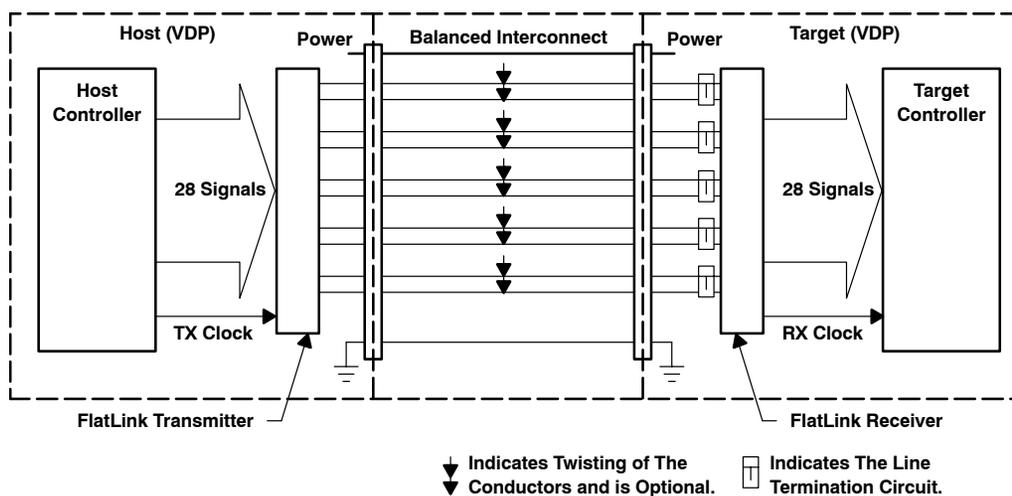
**Figure 1. Typical Connection of One FlatLink Transmitter and One Receiver.**
