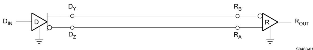
**Figure 16. Differential Unterminated Configuration**
