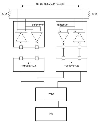
Figure 7-1. Experimental 2-Node CAN Bus
