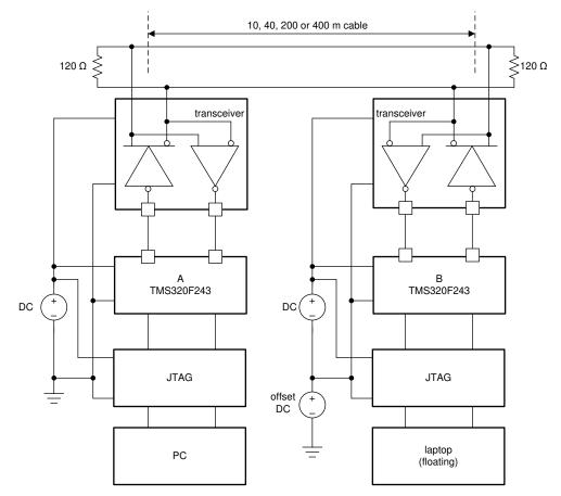
Figure 7-3. Experimental 2-Node CAN Bus With Offset Grounds
