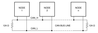
Figure 3-1. Multipoint Topology of a CAN Bus
