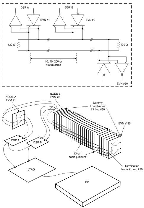
Figure 7-2. Experimental 30-Node CAN Bus
