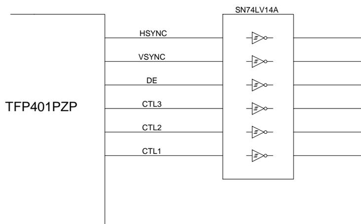
**Figure 5. Example Schmitt-trigger application**
