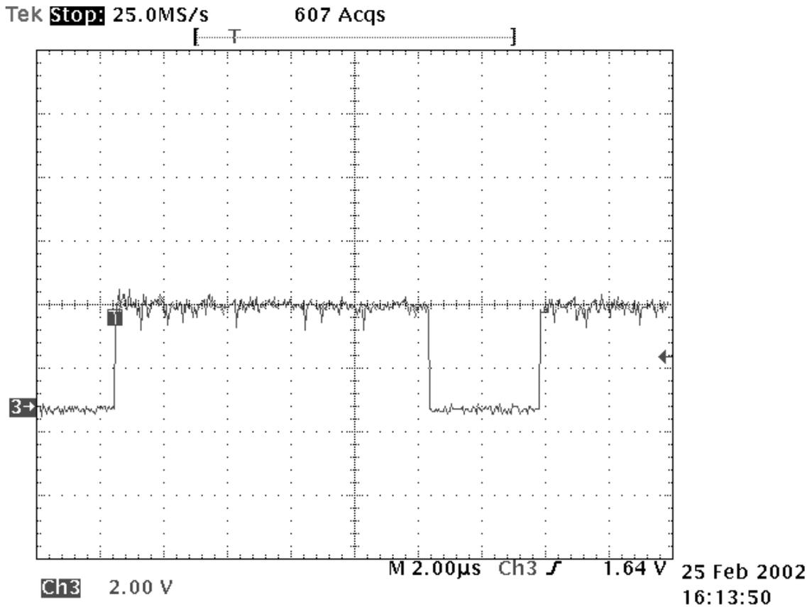
Figure 4. Example DE waveform TFP401 (2Pix/cik, STAG/=H, ST=L) UXGA resolution all outputs switching simultaneously.
