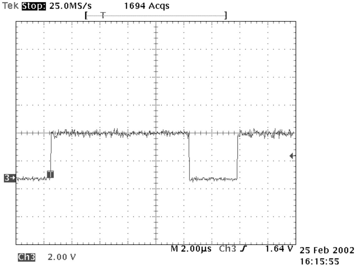
Figure 2. Example DE waveform TFP401 (2Pix/cik, STAG/=L, ST=L)
