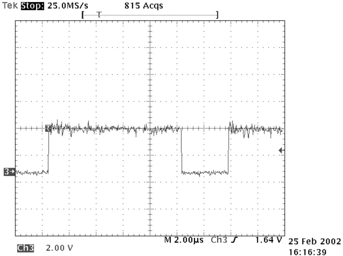
**Figure 3. Example DE waveform TFP401 (2Pix/cik, STAG/=L, ST=H)
