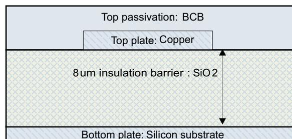
**Figure 1. Isolation Barrier for ISO72x Family of Products**
