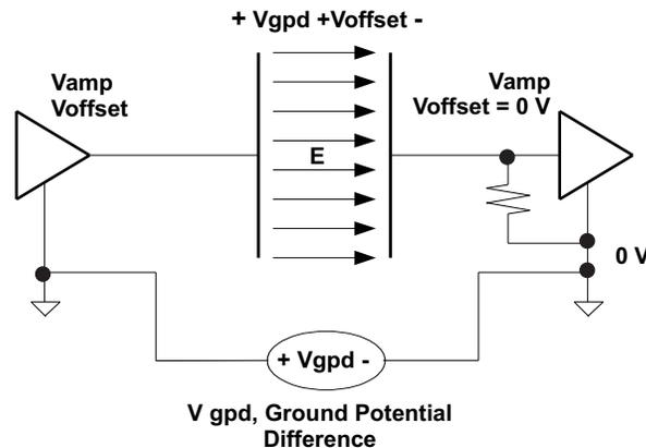
Figure 8. Capacitive Coupling
