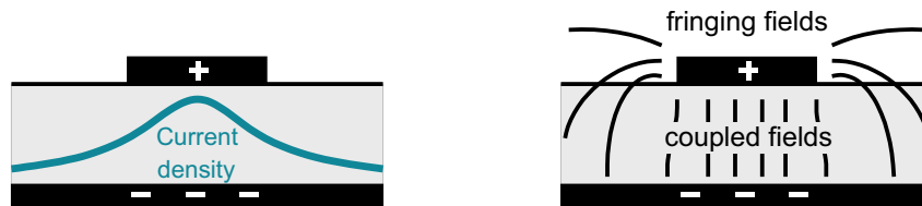
Figure 4-7. Ground Plane Acting as a Single Return Trace
