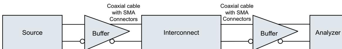
**Figure 8. Generic Test Setup – Two Buffers**
