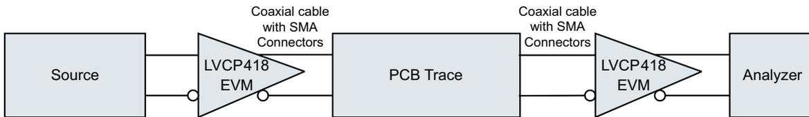
Figure 15. SN65LVCP418/PCB Trace Test Setup
