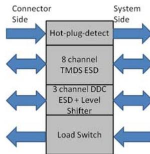
**Figure 1. Circuit Schematic**
