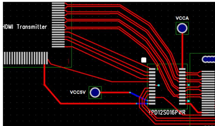
**Figure 8. TPD12S016PW routing with Type A Receptacle**
