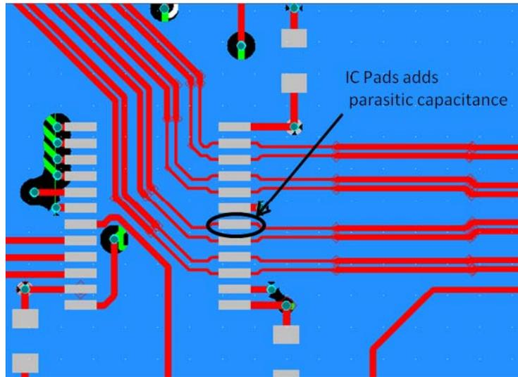
**Figure 13. Skinny traces for TMD5 lines**
