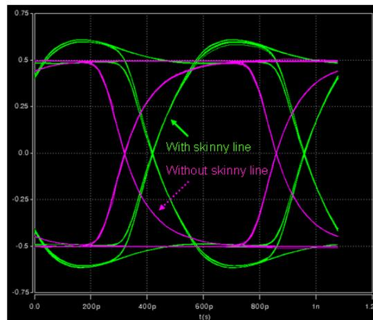
**Figure 14. Simulated Eye-diagrams with and without Skinny Traces**
