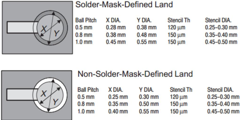
Figure 7. Recommended Land Pattern Configurations
