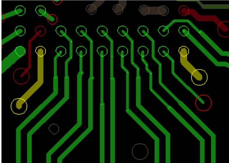
**Figure 1. DSI Channel Routing Example**
