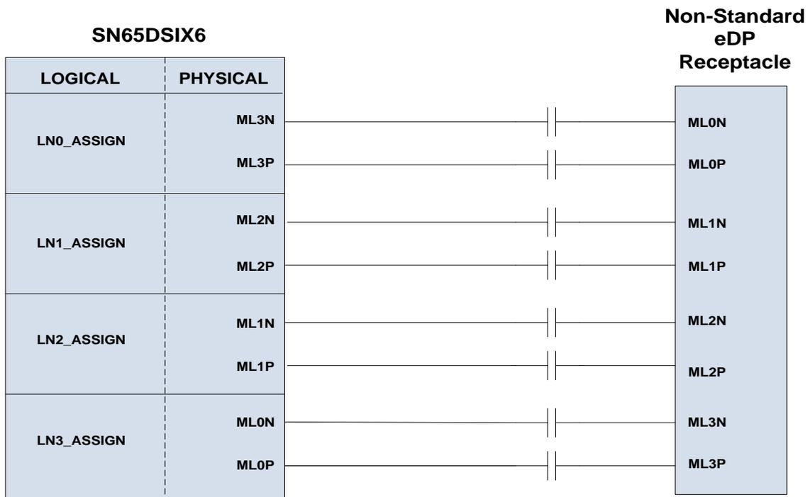
**Figure 3. Custom Lane Assignment Example**
