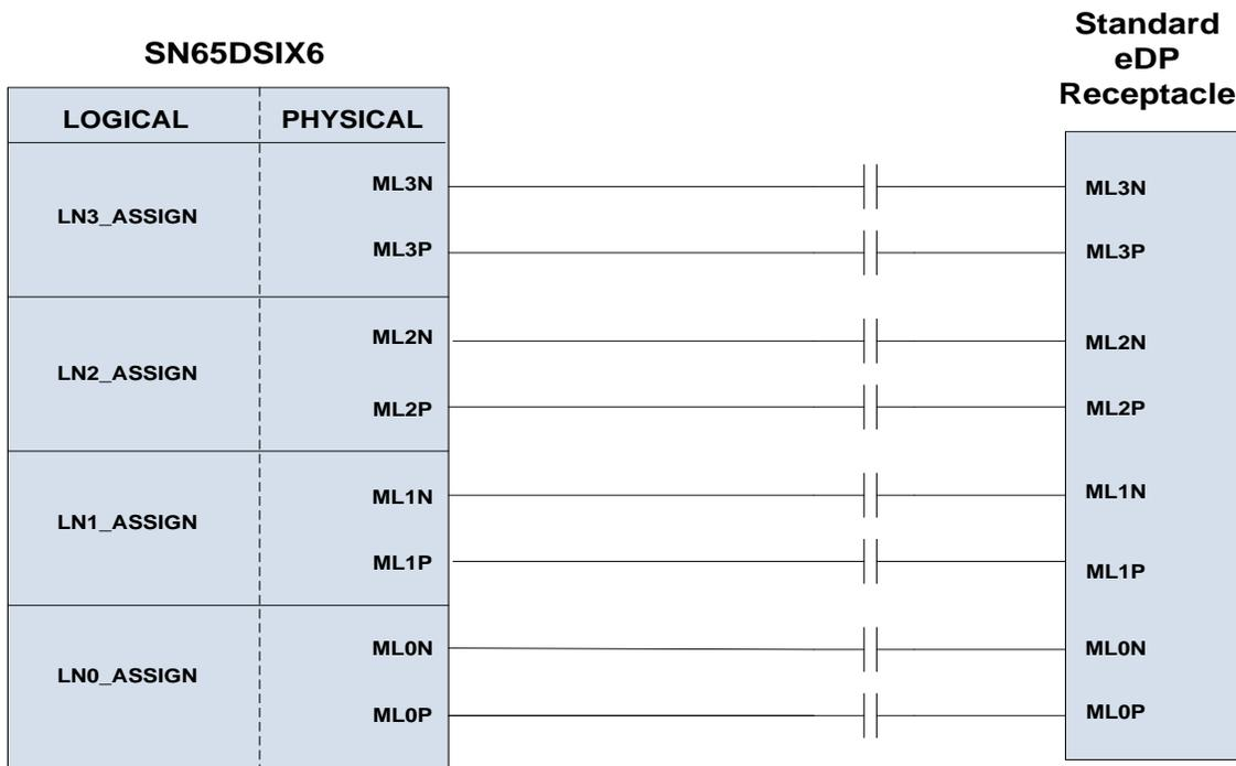
**Figure 2. Default Configuration Lane Assignment Example**
