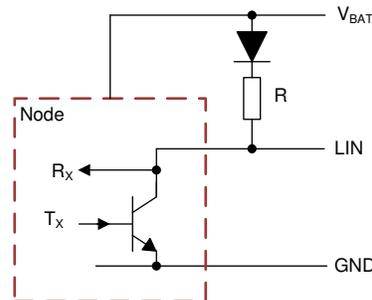
**Figure 3-1. Simplified LIN Driver Schematic**
