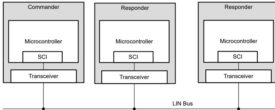
**Figure 2-1. High-Level LIN Transceiver in Network**
