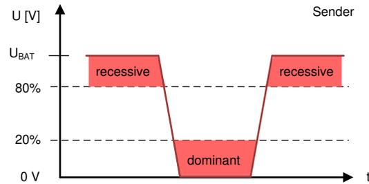
**Figure 3-2. Bus Signal Thresholds for Senders**
