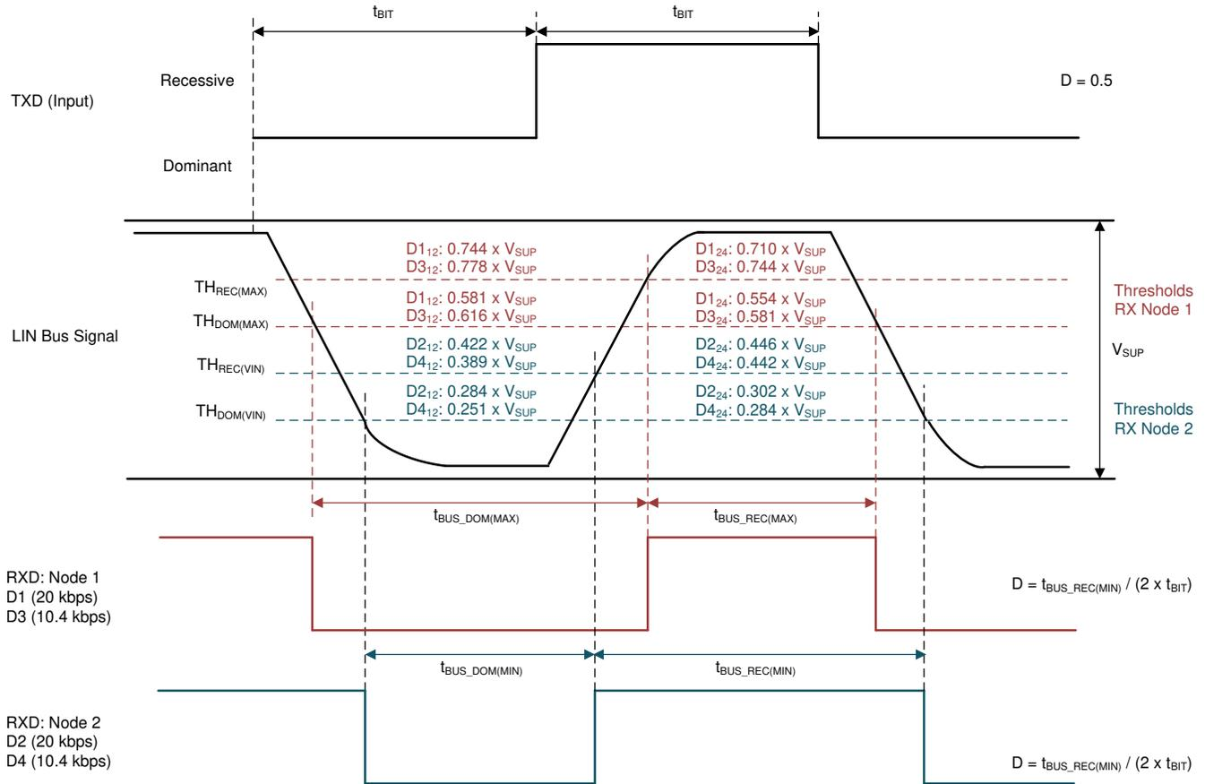
Figure 3-5. Bus Duty Cycle Requirement
