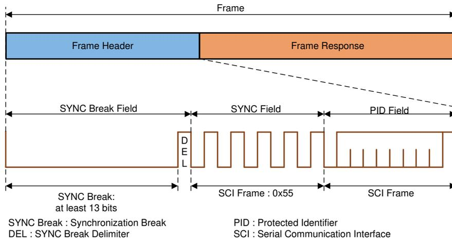
**Figure 2-2. LIN Frame Header Explanation**
