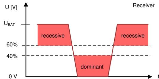
**Figure 3-3. Bus Signal Thresholds for Receivers**
