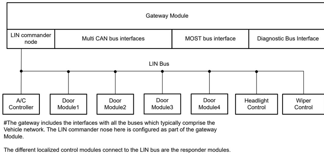
**Figure 1-1. High-Level Application Diagram**
